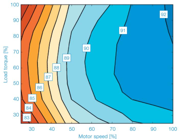
High output motor-drive package efficiency (40 kW, 1500 rpm)
