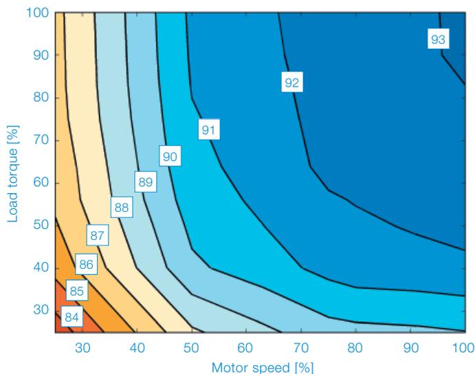
IE4 SynRM motor-drive package efficiency (37 kW, 1500 rpm)
