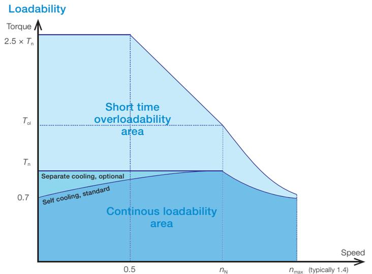
Torque characteristics of SynRM motors
