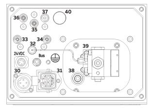
Figure 13: Gas and electric connections Fidas24 and Fidas24 NMHC
