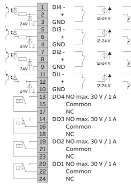
Image 21: Electrical connections, digital I/O module
