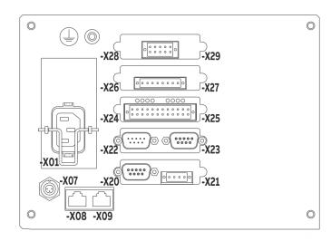
Image 18: Terminal assignment of electronic module (example)
