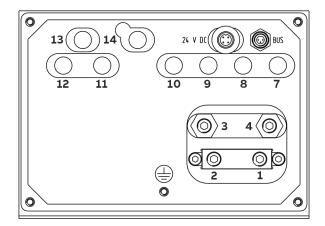
Figure 12: Gas connections Caldos27
