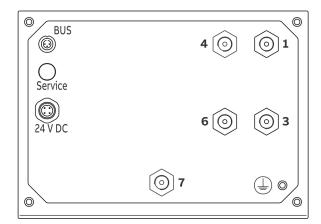
Figure 5: Gas connections Limas21 UV
