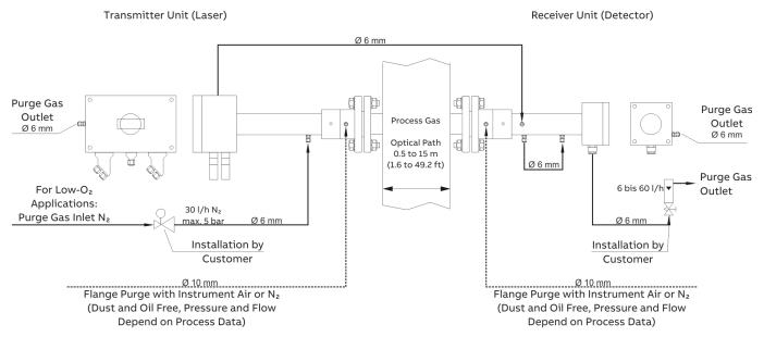
Figure 3: Purging of the transmitter and receiver units
