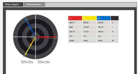
Vector diagram to control connections
