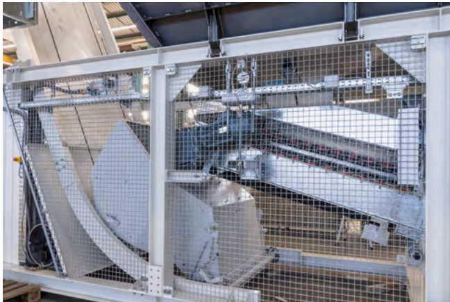
Metering via weighing belt into the skip bucket.
