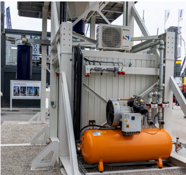
Compact mixing plant: Integrated compressed air system, water connection, pluggable electrical connection points for the linear bin and as option the warm water connection.
