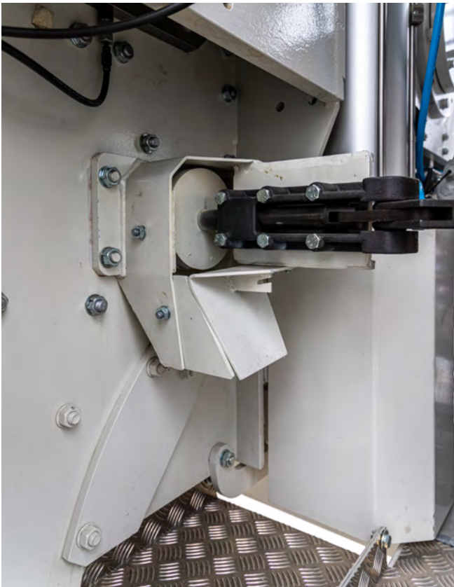
Optional concrete probe outlet mixer.
