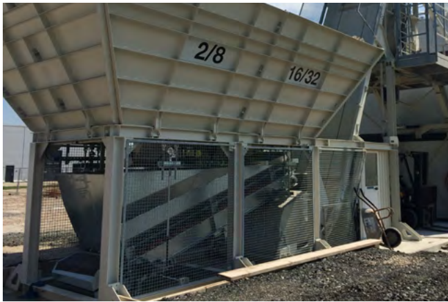
Compact linear bin with integrated weighing conveyor belt.
