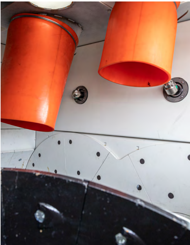
Mixer inlet for cement with the options silica inlet and mixer cleaning system.
