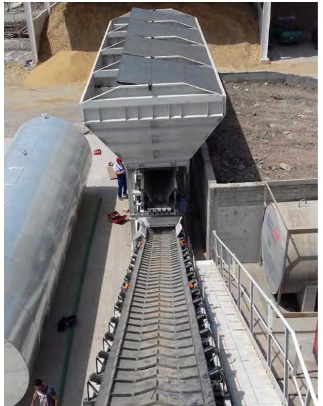
Chevron conveyor belt with optional walkway one-sided.
