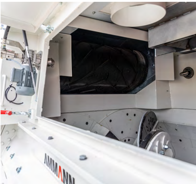
Aggregates transfer into the mixer trough conveyor belt.
