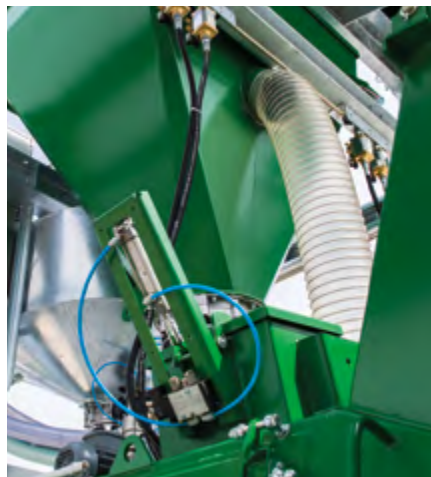
The mixer and cement weigher are connected via an aeration hose. The self-contained system ensures the required pressure compensation.
