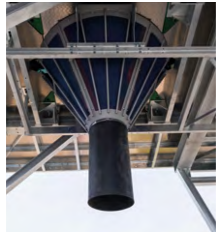
Lowerable mixer discharge funnel clad with EWP wear protection.
