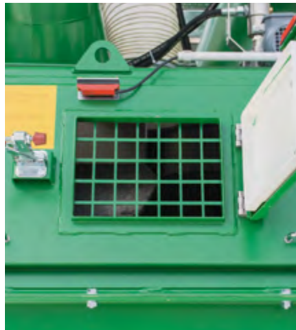
Mixer viewing window: a safety end switch ensures visual control when the mixer cleaning system is switched on.
