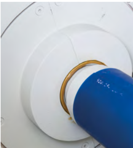
The half-shelf on the shaft sealing enables quick and easy maintenance. It is no longer necessary to remove the gear system and motor.
