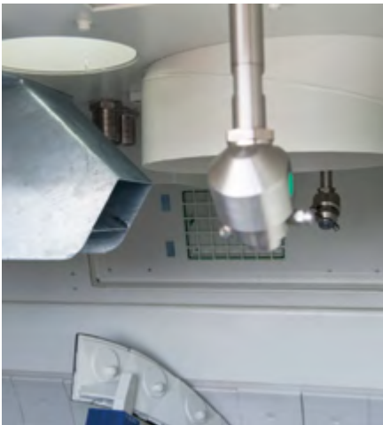
A total of four motorised cleaning jets ensure the mixer looks as good as new.
