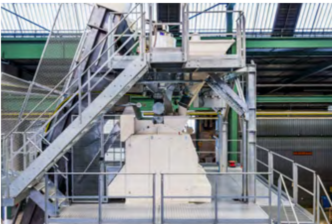
Optional extendable mixer platform for individual execution.
