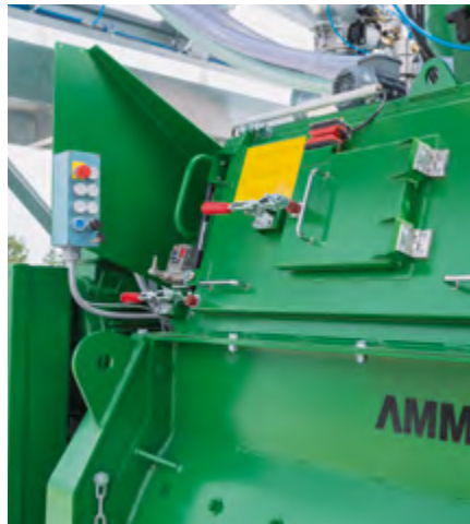
Local mixer operation facilitates cleaning and maintenance work.
