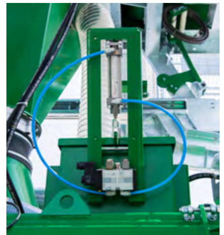
Quality control via optional camera system: mounted to a pneumatically operated camera shaft directly on the mixer.
