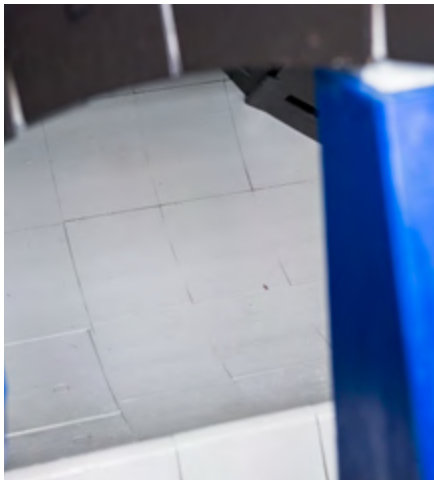
The mixer wearing parts consist entirely of screwless elements. Only the two last rows are screwed into place. The big advantage: better utilisation of wear material.
